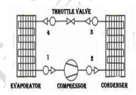
**Figure 1:** Schematic diagram of air-source heat pump valve.
